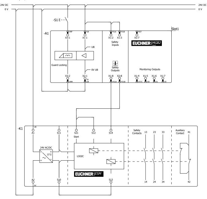
Figure 1: Basic circuit diagram (shown with the ESM-BA301)
