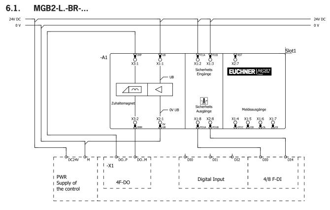
Figure 1: Basic circuit diagram, MGB2-L.-BR-...
