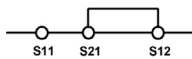
Fig. 12: Automatic start. Max perm. delay during closing of the safety switches on S12 and S13: S12 before S13: 300 ms S13 before S12: any
