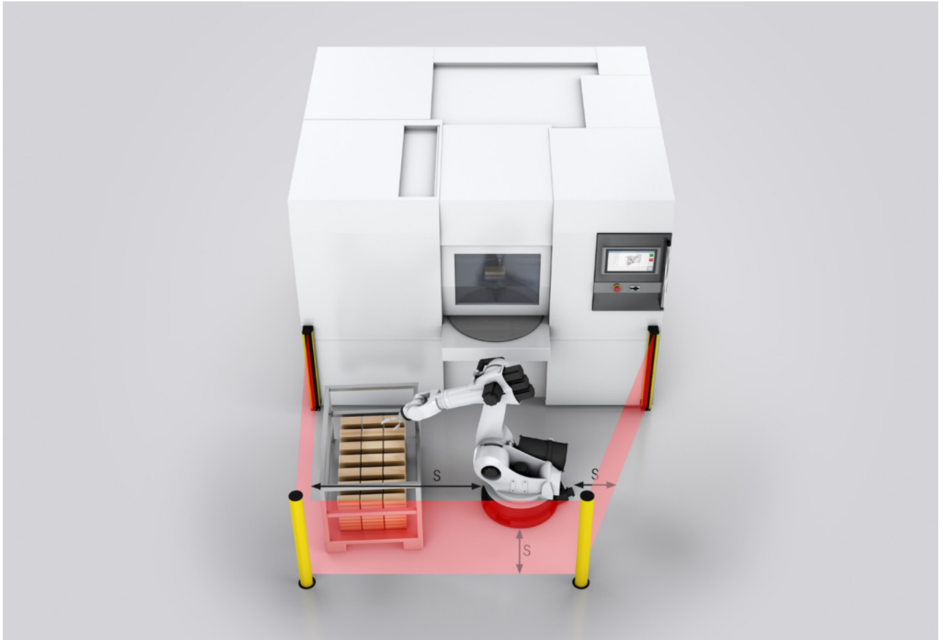
Figure 5: Safety distance S
