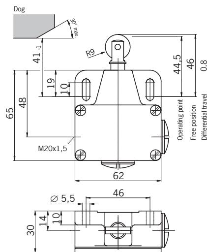
Fig. 7: Dimension drawing for N11 with extended roller plunger
