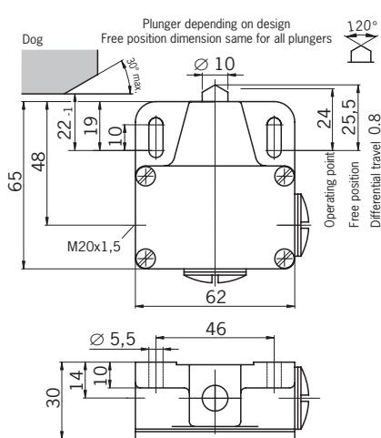
Fig. 6: Dimension drawing for N11
