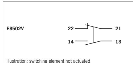
Fig. 2: Switching element and terminal assignment
