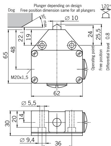
Fig. 4: Dimension drawing for N10
