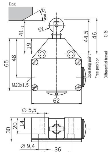
Fig. 5: Dimension drawing for N10 with extended roller plunger
