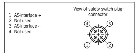
Figure 2: Terminal assignment, AS-Interface M12 plug connector
