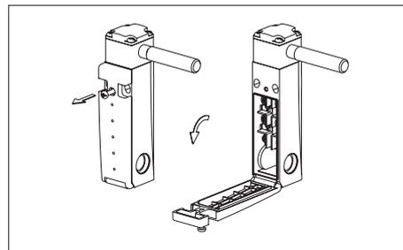
Fig. 2: Opening the safety switch
