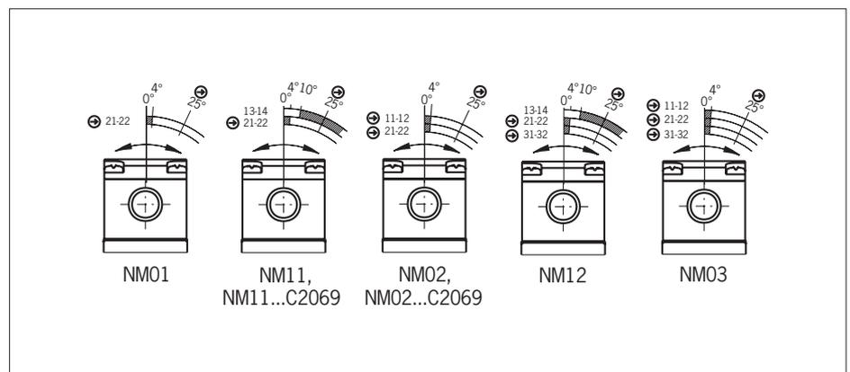
Fig. 4: Travel diagrams for NM..AV/NM..AL
