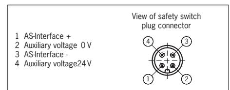
Fig. 5: Terminal assignment of M12 plug connector
