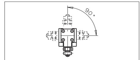
Fig. 3: Horizontal adjustment
