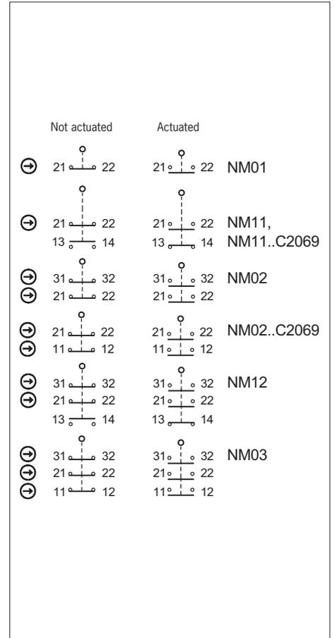
Fig. 7: Switching elements and switching functions
