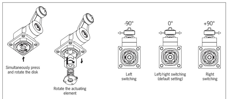
Fig. 4: Changing the switching direction
