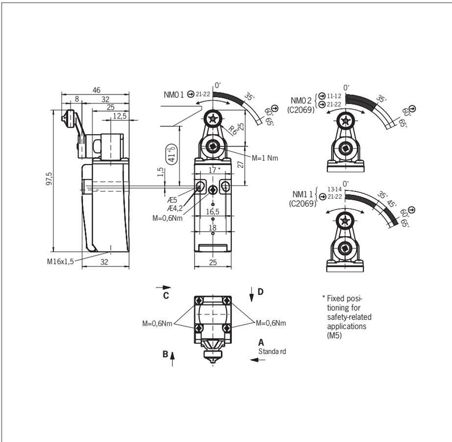
Fig. 6: Dimension drawing and travel diagrams for NM01HB, NM...C2069
