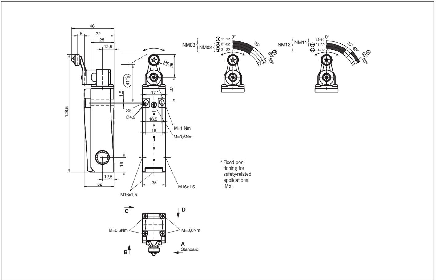
Fig. 5: Dimension drawing and travel diagrams for NM11HB / NM02HB / NM12HB / NM03HB
