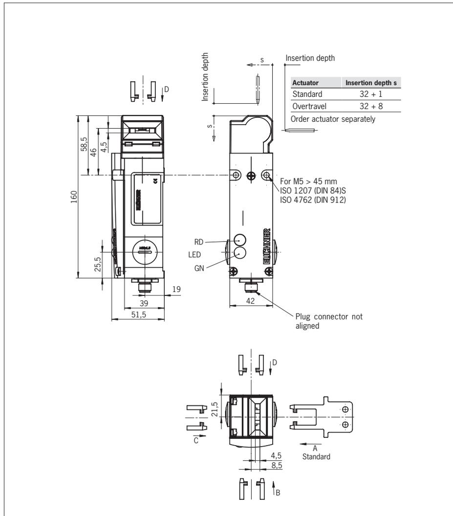
Fig. 4: Dimension drawing for NX...AS
