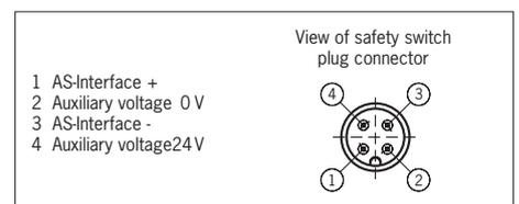
Fig. 3: Terminal assignment of M12 plug connector
