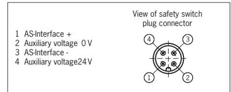
Fig. 2: Terminal assignment of M12 plug connector
