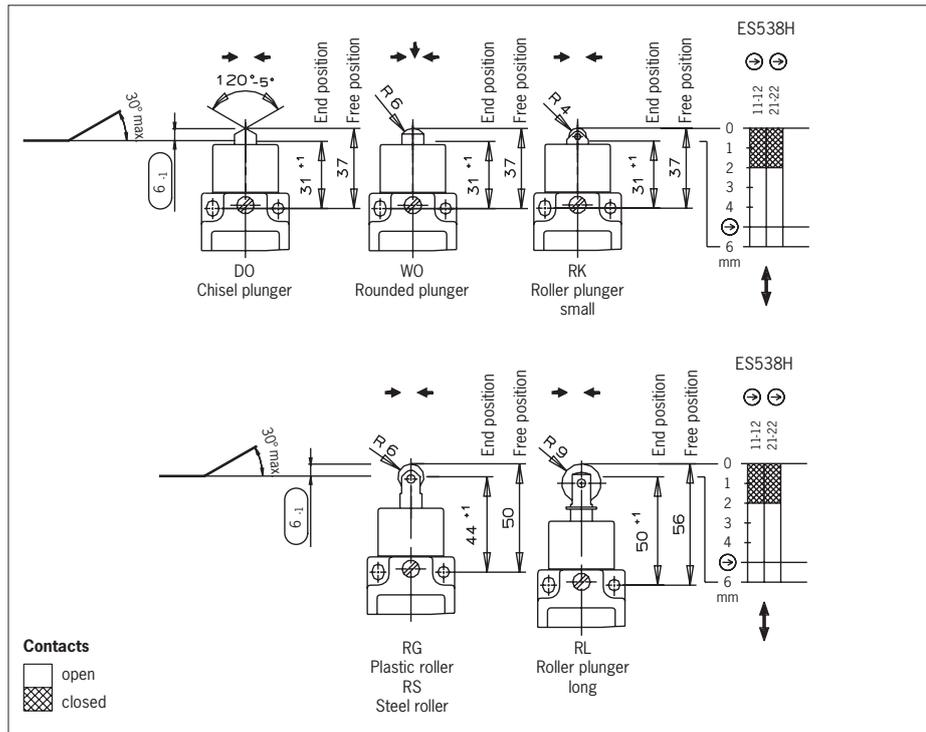
Fig. 4: Travel diagrams, actuator and approach directions
