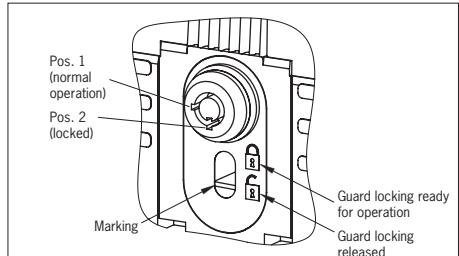
Fig. 1: Auxiliary key release and indication
