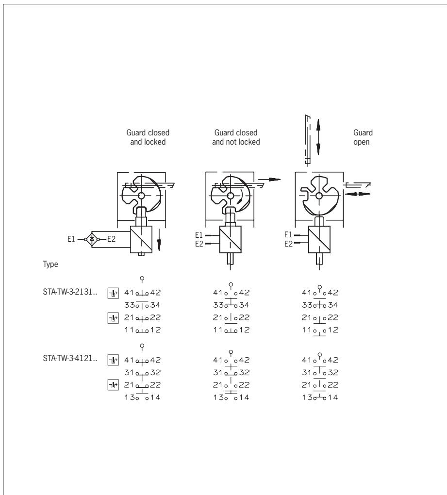
Fig. 3: Switching elements and switching functions
