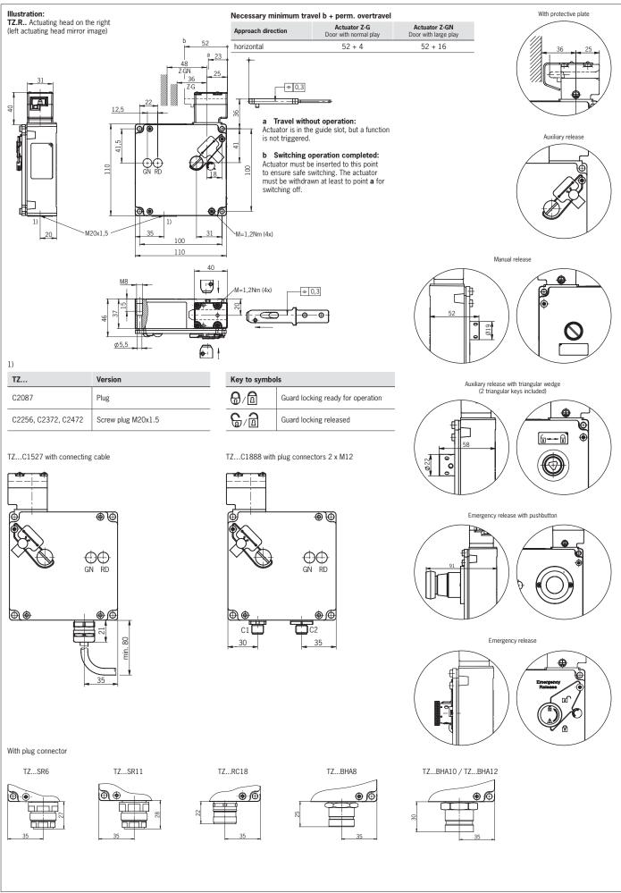
Fig. 3: Dimension drawing for TZ...
