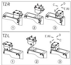
Fig. 2: Changing the actuating direction
