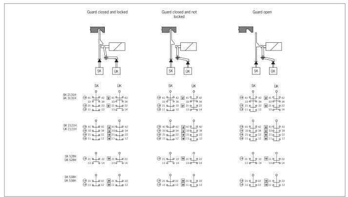
Fig. 5: Switching elements and switching functions
