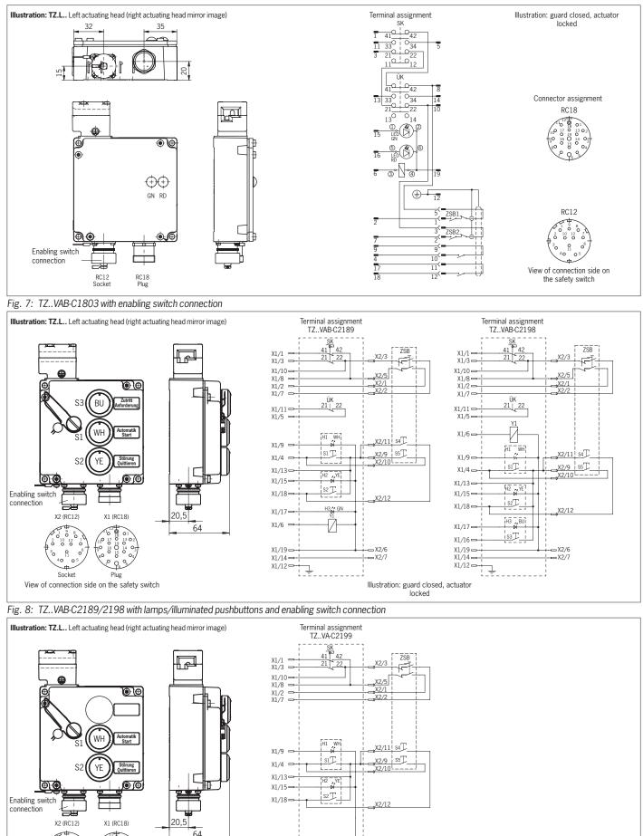
Fig. 9: TZ..VA-C2199 with illuminated pushbuttons and enabling switch connection
