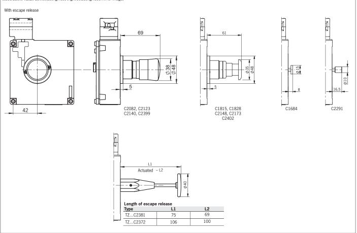
Fig. 4: Dimension drawings for escape releases
