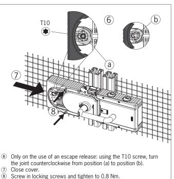
Fig. 13: Changing actuating direction, steps 6 to 8
