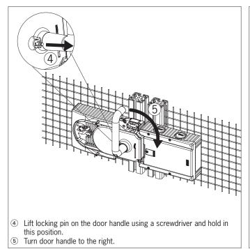
Fig. 12: Changing actuating direction, steps 4 and 5
