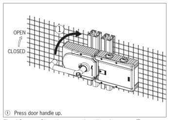
Fig. 10: Changing actuating direction, step ①
