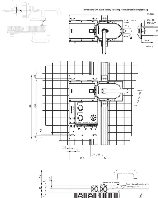
(Figure shows version for doors hinged on the right, pre-assembled on mounting plates)
