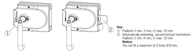
Fig. 7: Lockout mechanism secured with padlock
