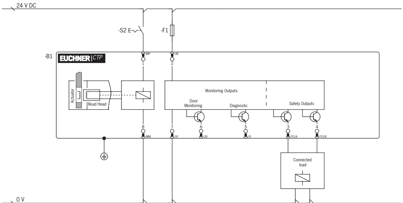
Figure 3: Connection example, version with plug connector M12
