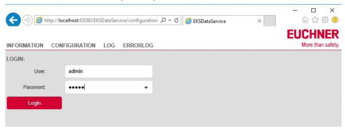
Only one user can be logged in using the service at a time. If another user logs in via another computer, the first user will be logged out automatically.
