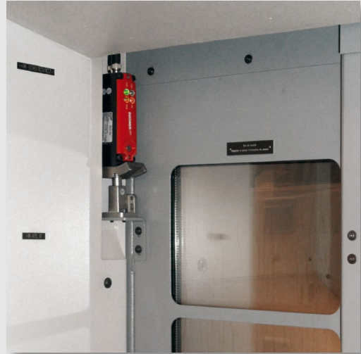
Securing a sliding door
