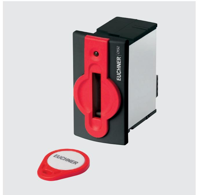
The new key system CKS2 consists of a key adapter and highly coded keys with transponder technology. The device safely detects whether a specific key is inserted or not. If there is a key in the key adapter, the data on the key are read and checked for validity. If the key is recognized as valid, the safety outputs are switched on. One key can be assigned to several key adapters in different installations.
