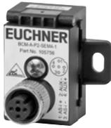
For connection of components with integrated AS-Interface and M12 plug connector to the AS-Interface ribbon cables. Both the bus and auxiliary power are converted from the ribbon cable to an M12 socket. The coupling module is suitable for safety components and for standard components. It is particularly suitable for EUCHNER safety switches with guard locking.
