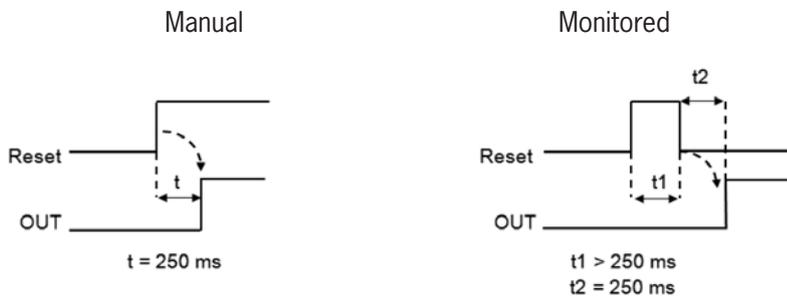
Figure 89: Interlock manual/monitored reset
