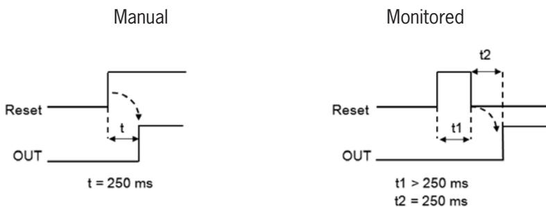
Figure 86: Emergency stop manual/monitored reset
