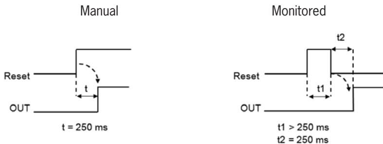
Figure 101: Safety footswitch manual/monitored reset
