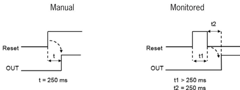
Figure 105: Light barrier manual/monitored reset
