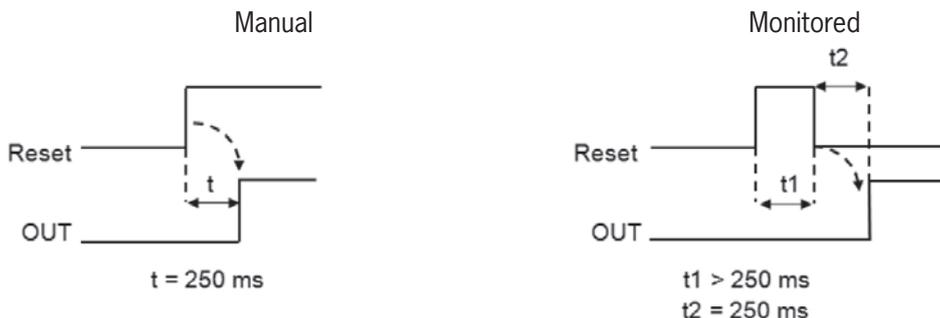
Figure 92: Single-channel interlock manual/monitored reset
