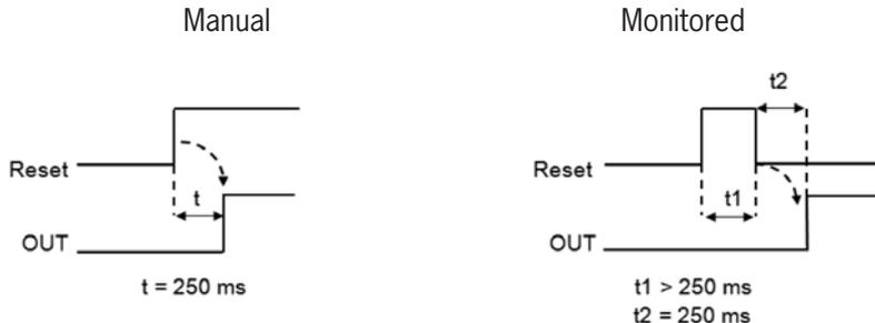
Figure 98: ESPE manual/monitored reset
