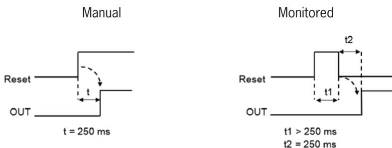
Figure 112: Pressure sensitive mat manual/monitored reset
