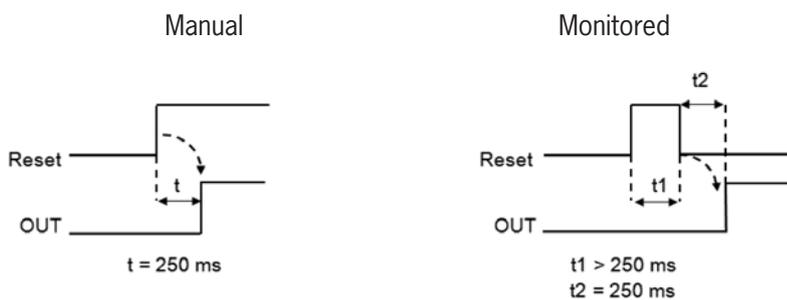
Figure 95: Key-operated rotary switch manual/monitored reset
