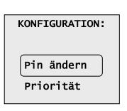
A selection is made using the  $\P$  keys, the selection is confirmed using <ENTER>. The Configuration (Konfiguration) menu is left using the <ESC> key.
