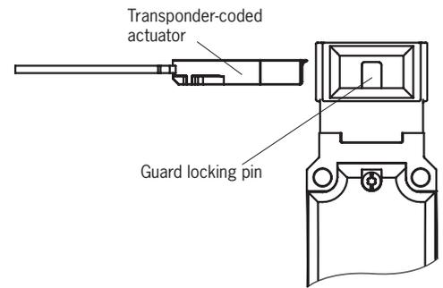
When the guard is closed, the actuator is moved into the safety switch. When the operating distances are reached, power is supplied to the actuator by the switch and data are transferred.
