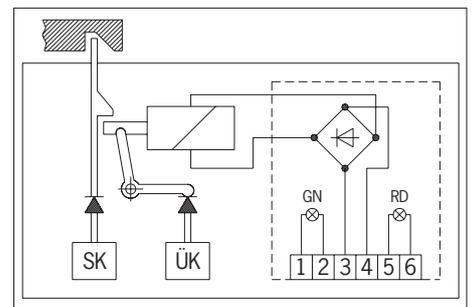
Fig. 1: Function of safety switch TZ
