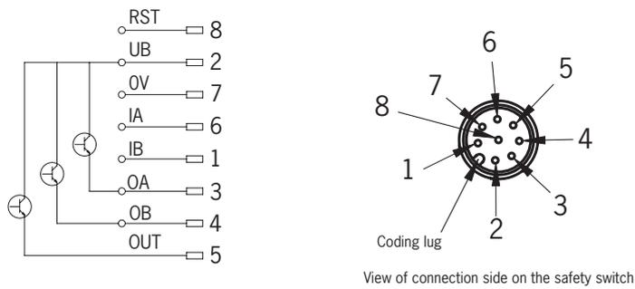
Figure 2: Connector assignment of safety switch CES-AR
