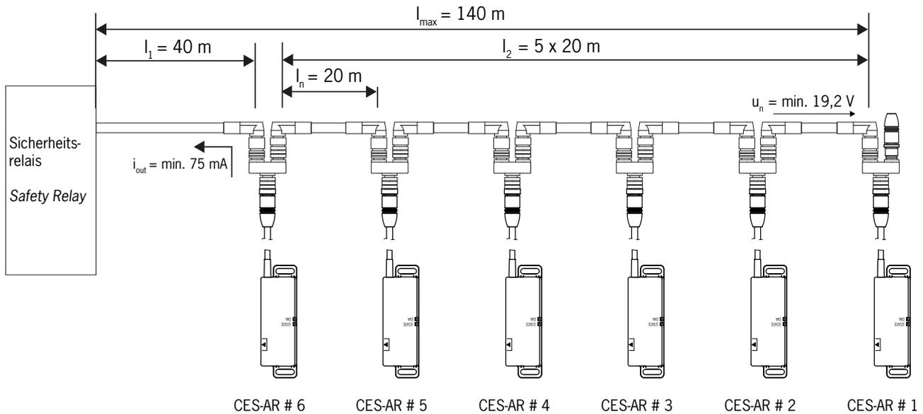
Figure 1: Circuit example with six CES-AR
