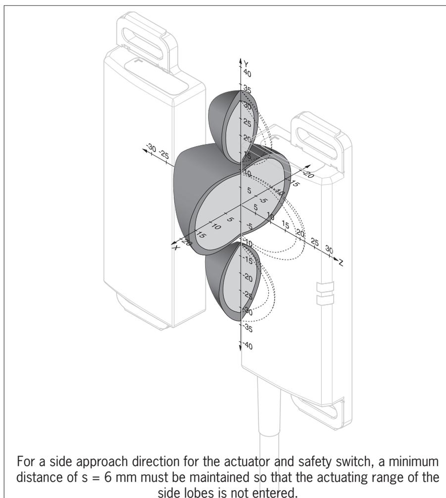
Figure 6: Typical actuating range
