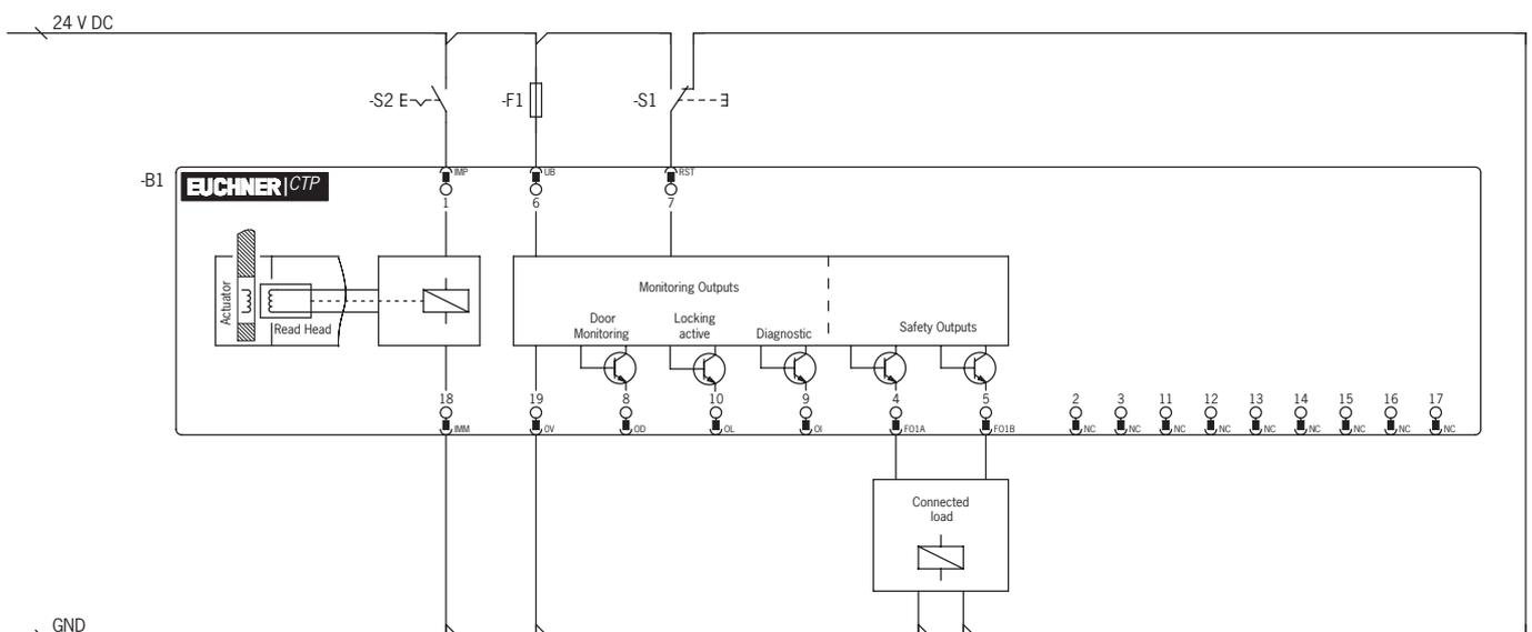
Figure 3: Connection example, version with plug connector M23
