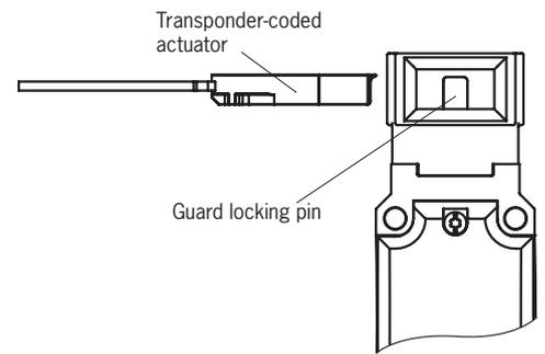
When the guard is closed, the actuator is moved into the safety switch. When the operating distance is reached, power is supplied to the actuator by the switch and data are transferred.
