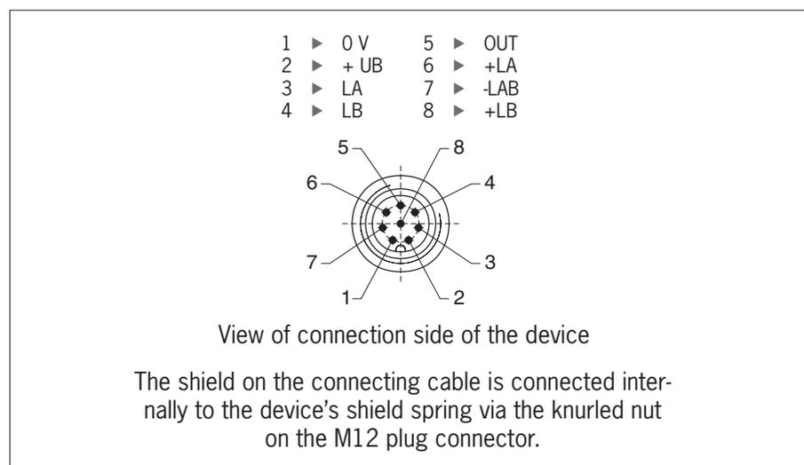
Fig. 1: Connector assignment of safety switch CES-A-C5H-01-EX
