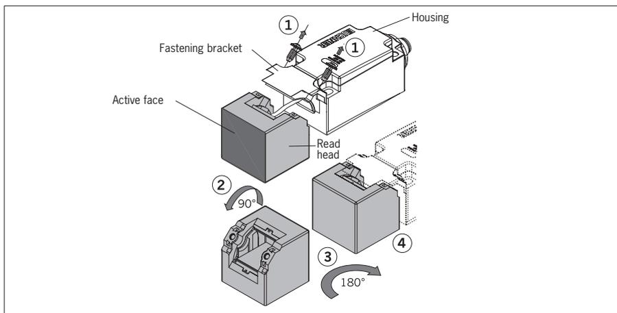
5. Remove the clip from the underside of the housing to change the lateral approach direction.
