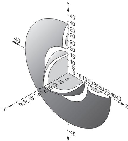
For a side approach direction for the actuator and read head, a minimum distance of  $s = 6$  mm must be maintained so that the actuating range of the side lobes is not entered.
