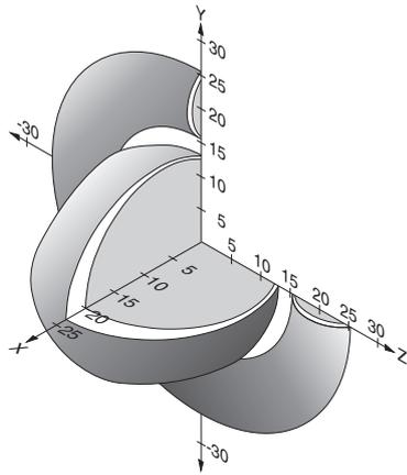
For a side approach direction for the actuator and safety switch, a minimum distance of  $s = 4$  mm must be maintained so that the actuating range of the side lobes is not entered.
