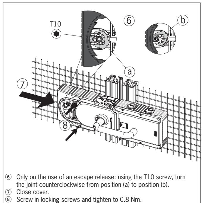
⑥ Only on the use of an escape release: using the T10 screw, turn the joint counterclockwise from position (a) to position (b).
