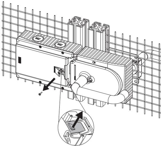
Fig. 6: Auxiliary release
