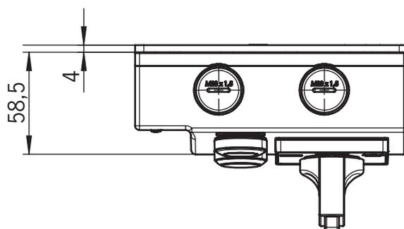
**Control module MGB-CB-...-PN on mounting plate**
