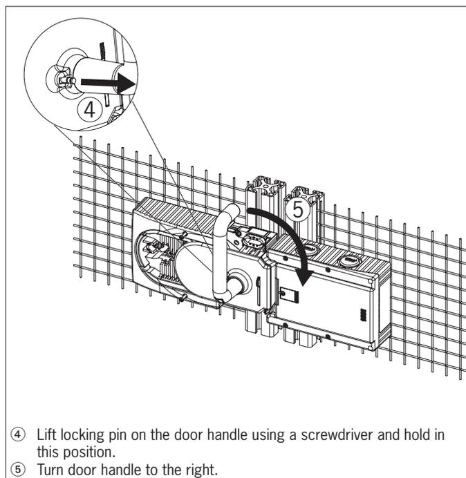
④ Lift locking pin on the door handle using a screwdriver and hold in this position.
