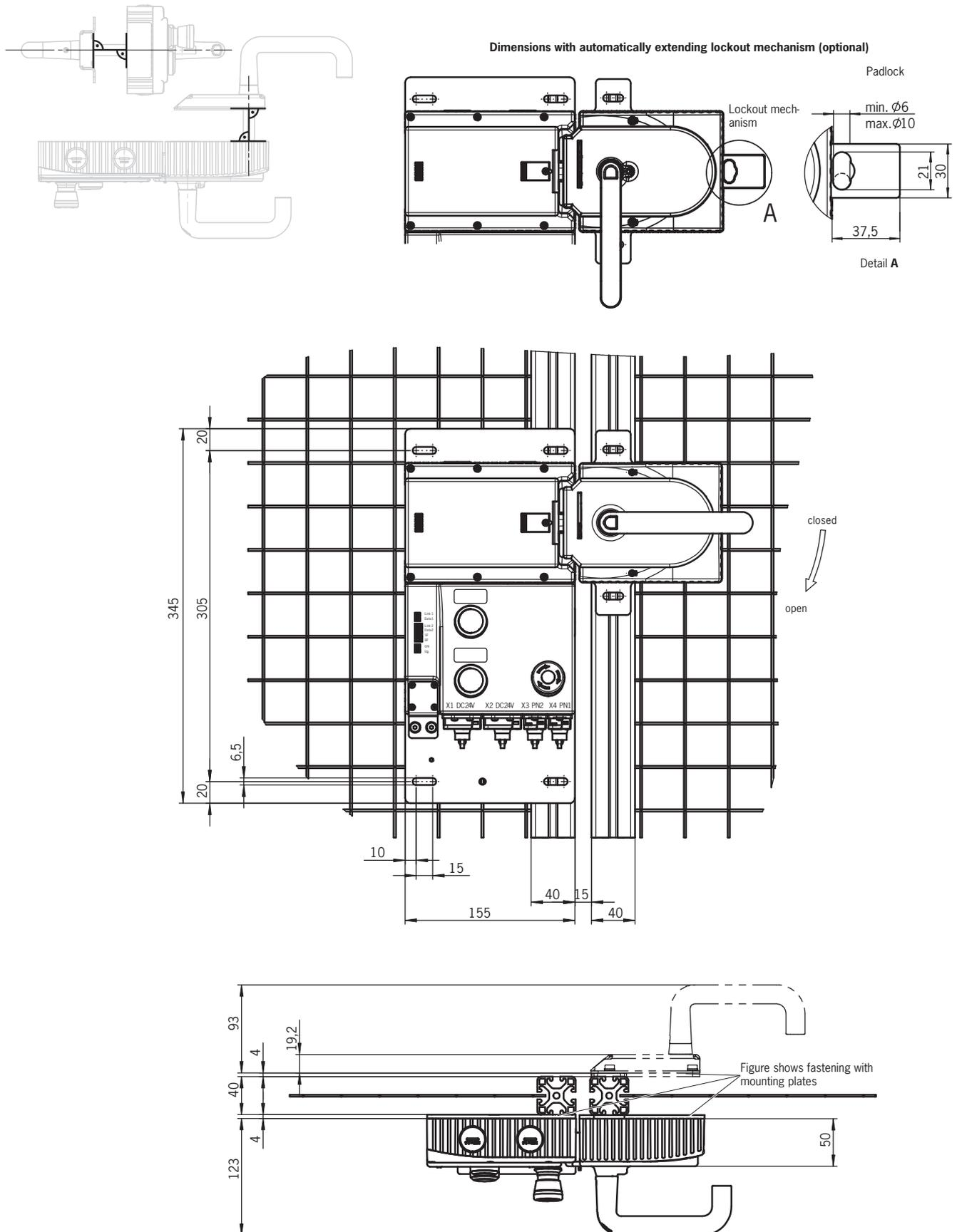
(Figure shows version for doors hinged on the right, pre-assembled on mounting plates)
