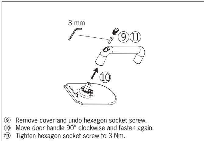
Fig. 14: Changing actuating direction, steps ⑨ to ⑪
