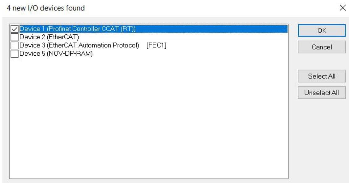
Figure 4: Selection of PROFINET controller
