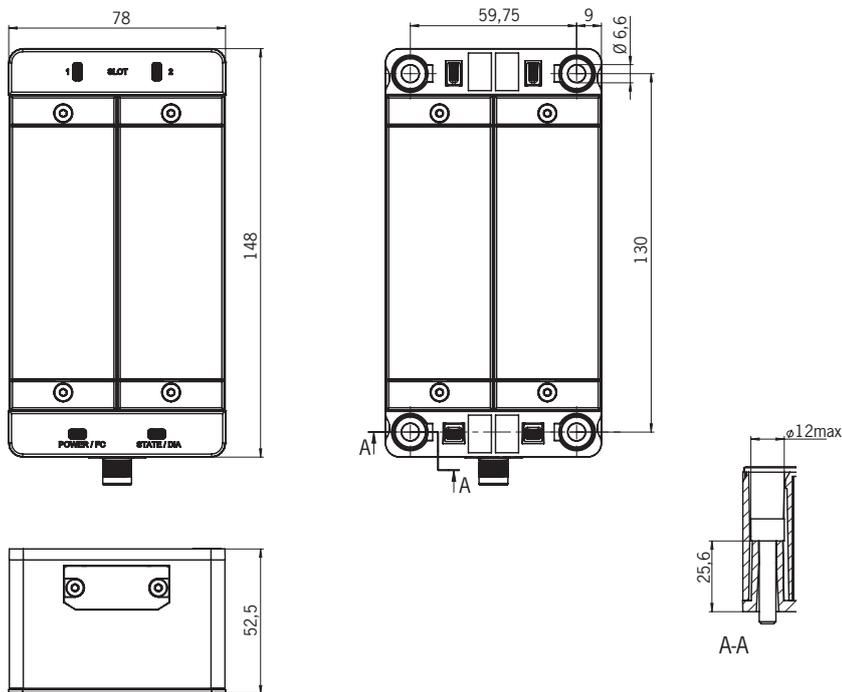
Fig. 4: Dimension drawing for 2-slot expansion module MCM
