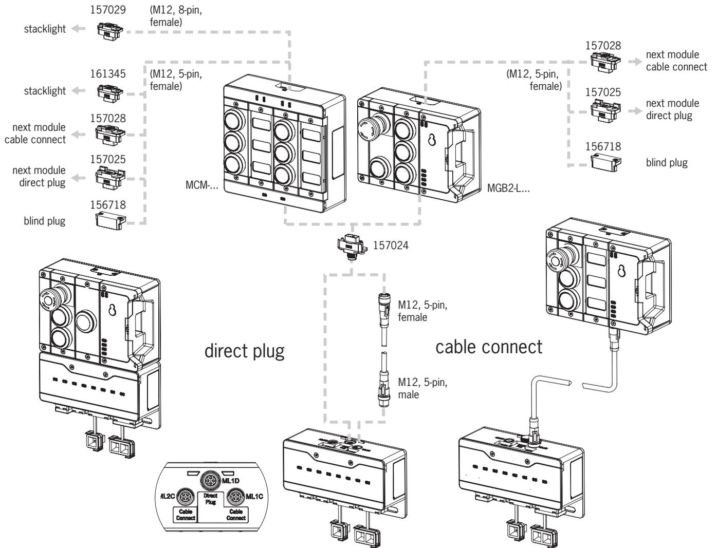
Fig. 6: Connecting modules
