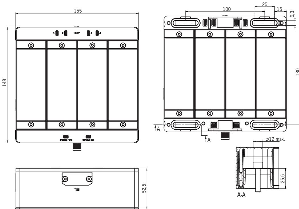
Fig. 3: Dimension drawing for 4-slot expansion module MCM
