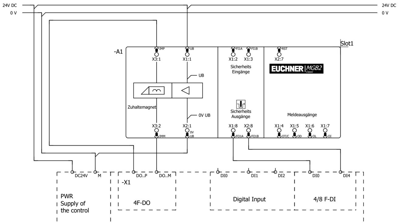
Figure 2: Basic circuit diagram, MGB2-L.-BP-...
