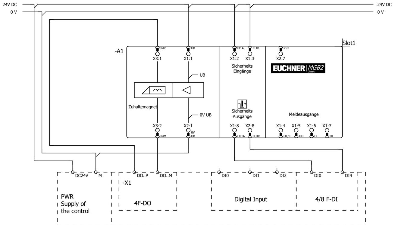
Figure 1: Basic circuit diagram, MGB2-L.-BR-...
