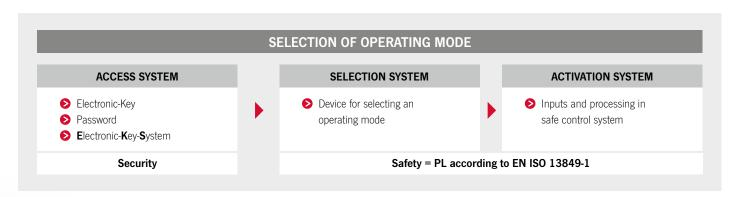
The access system does not have to be implemented according to EN ISO 13849-1. It is not possible to determine a PL for the monitoring of an authorization. By contrast, the selection system and the safe control system of a machine must fulfill the required PL.
