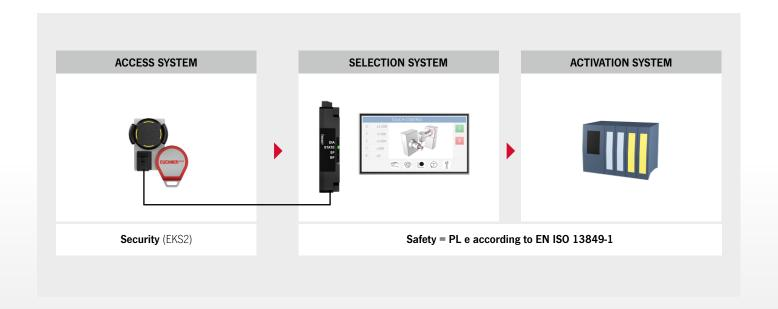
The PL calculation is more difficult if a touchscreen is to be used as the selection system, because a touchscreen does not represent a safe selection system and there are no available values for the PL calculation. The EKS2 from EUCHNER now permits selection of operating mode via a touchscreen to be implemented up to PL e.
