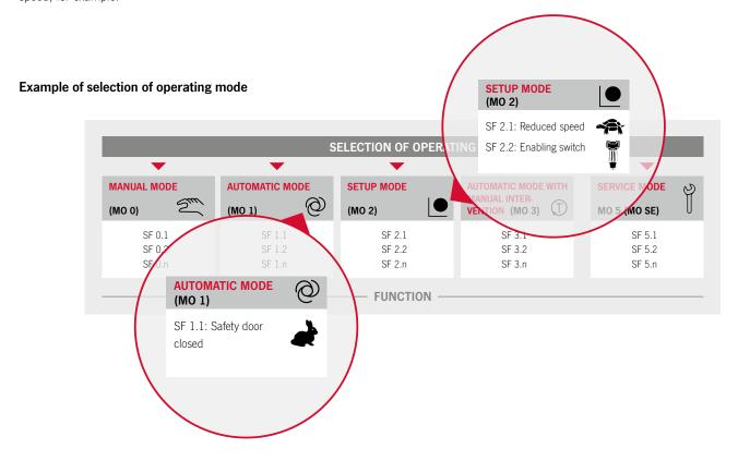
Changing the operating mode switches from one safety system to another one. Improper switchover can endanger the operator, so selection of safe operating mode must fulfill a Performance Level according to EN ISO 13849-1 corresponding to the risk assessment of the machine/installation.
